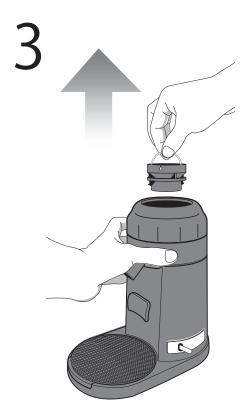
Lift out the top burr from the grind adjustment collar using the handle. Clean using the burr cleaning brush.
