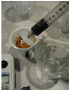
Attach a syringe filter approx a quarter-turn until snug. Do not over tighten.
