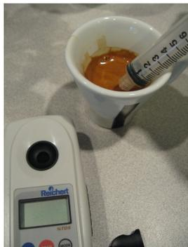
Allow 1 minute for espresso to cool and CO<sub>2</sub> to diffuse out of solution. Stir the sample.
