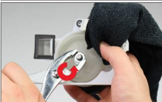
Push the driveshaft through the gear. A screwdriver handle generally works to hammer the shaft down and out of the gearbox.
