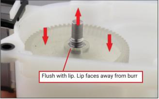
\*If having difficulty getting flush, make sure paddle wheel pegs are still indexed into cone burr. You can use your old cone burr as a block to help apply pressure with two hands to the drive gear if needed\*
