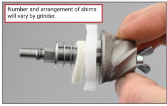
\*If the various shims were not kept separate, reference the GB2.0 guide for help re-arranging them\*
