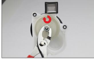
Attach the motor/motor plate to the gearbox. Tighten screws in a X pattern.
