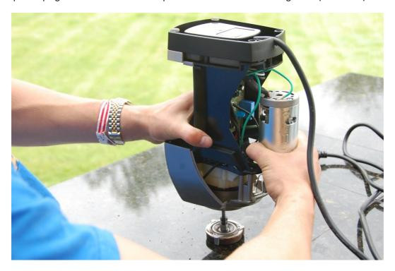
Flip the unit back upright. Pinch the drive belt and pull firmly to remove the belt and large pulley. Replace belt. TAKE NOTE that there is a lip on one edge of the large pulley. This lip should be on the bottom side.
