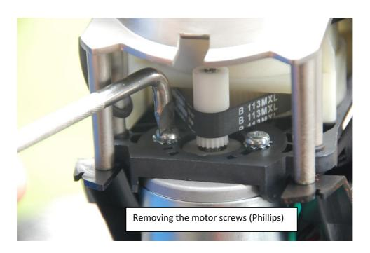
After removing the motor, hold the motor in one hand while flipping over the grinder with the other. A quick rap against the counter will drop the lower burr out from the grinder (see below)
