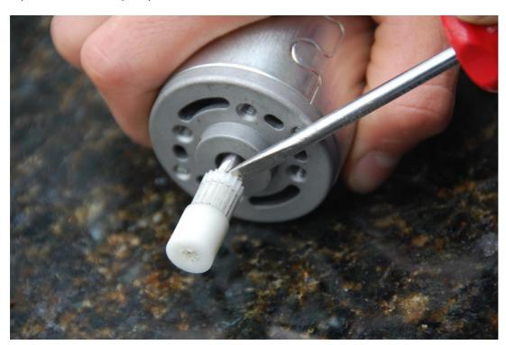
Replace with the new pulley. Make sure when the set screw is installed that it sits in the 'valley' of the helical motor shaft and not on one of the 'ridges', otherwise when you start the machine the screw will fall off of the 'ridge' and the pulley will no longer be secured.
